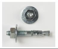
Wedge Anchors are a four-piece assembly consisting of an anchor bolt threaded at one end with a unified pitch, and a shoulder at the opposite end which retains a free-spinning clip. Each bolt comes with one nut and one washer. For use in solid based concrete, brick, or stone.
